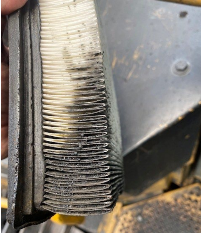
Filter breakthrough due to poor sealing
