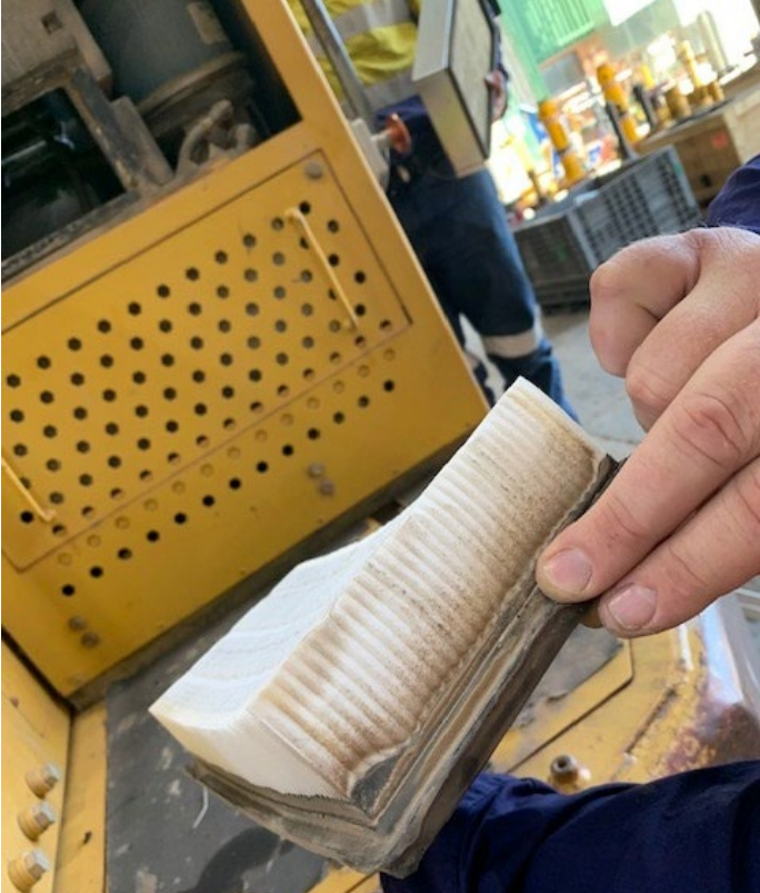
Poor sealing. Dust bypassing filter
