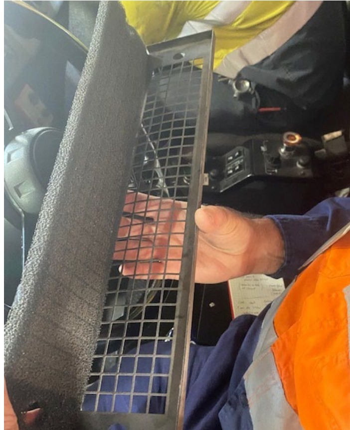
Non compliant coarse filter
