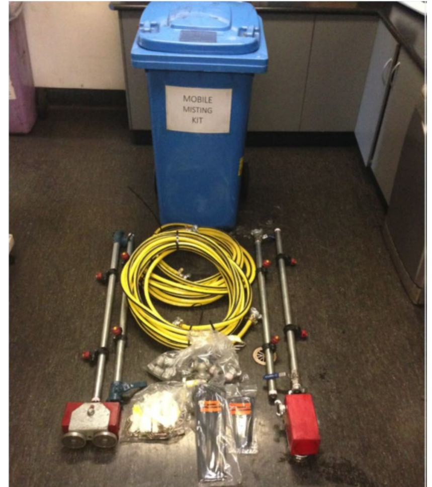
Mobile Misting Kit for Temporary Use in Case Other Controls Fail
